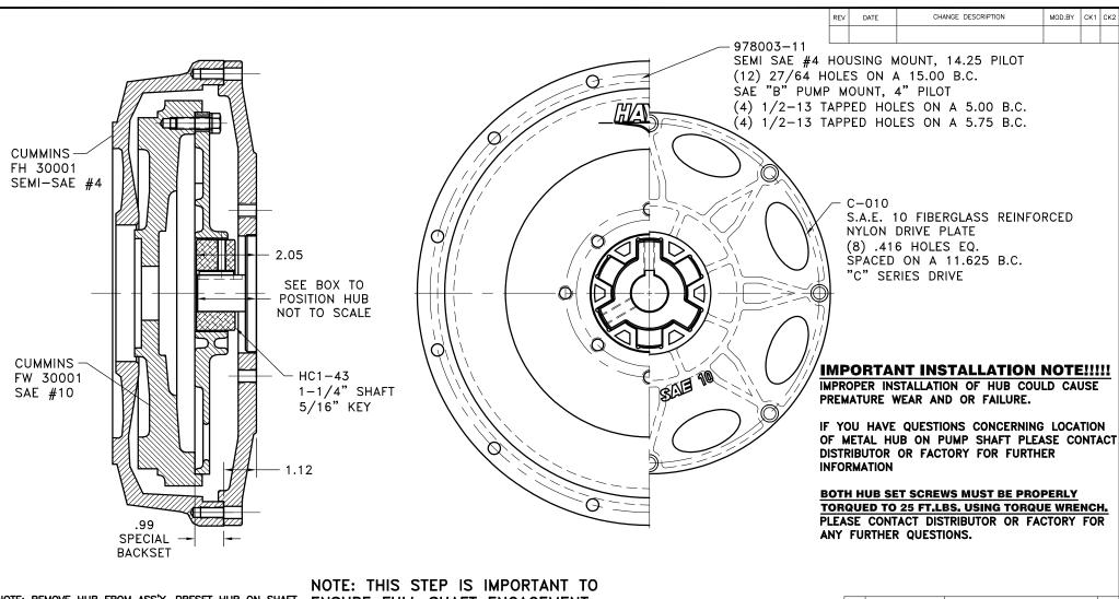
NOTE: REMOVE HUB FROM ASS'Y, PRESET HUB ON SHAFT AS SHOWN. TORQUE BOTH SET SCREWS TO 25 FT.LBS. USING TORQUE WRENCH. SHAFT SHOULD HAVE A MINIMUM OF 3/4" OF ENGAGEMENT IF NOT CONTACT FACTORY FOR RECOMMENDATIONS (231) 879-3372 TO GET HUB PRESET USE THIS EQUATION:
