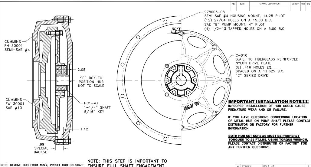
AS SHOWN. TORQUE BOTH SET SCREWS TO 25 FT.LBS. USING TORQUE WRENCH. SHAFT SHOULD HAVE A MINIMUM OF 3/4" OF ENGAGEMENT IF NOT CONTACT FACTORY FOR RECOMMENDATIONS (231) 879-3372 TO GET HUB PRESET USE THIS EQUATION:
