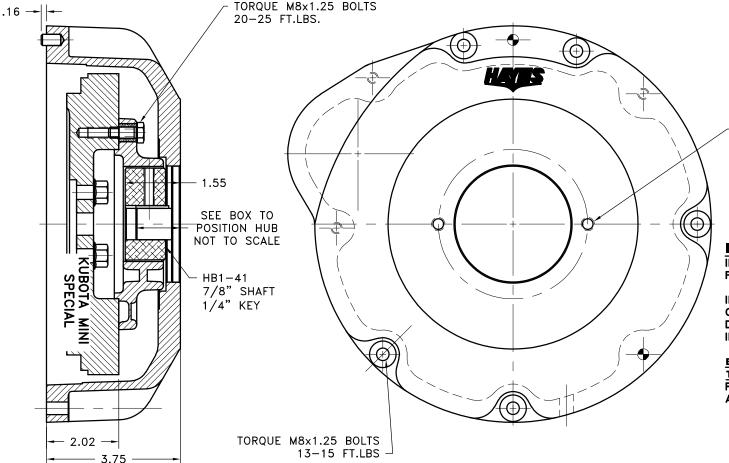
NOTE: REMOVE HUB FROM ASS'Y, PRESET HUB ON SHAFT AS SHOWN. TORQUE BOTH SET SCREWS TO 25 FT.LBS.
