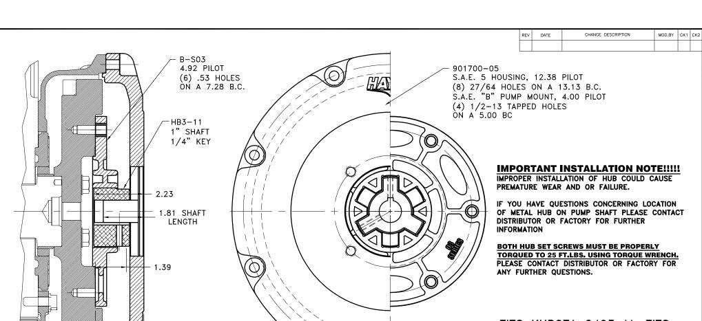
NOTE: REMOVE HUB FROM ASS'Y, PRESET HUB ON SHAFT AS SHOWN. TORQUE BOTH SET SCREWS TO 25 FT.LBS. USING TORQUE WRENCH. SHAFT SHOULD HAVE A MINIMUM OF 3/4" OF ENGAGEMENT IF NOT CONTACT FACTORY FOR RECOMMENDATIONS (231) 879–3372 TO GET HUB PRESET USE THIS EQUATION:
