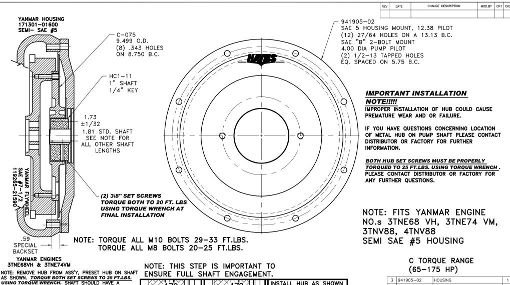
AS SHOWN. TORQUE BOTH SET SCREWS TO 25 FT.LBS. USING TORQUE WRENCH. SHAFT SHOULD HAVE A MINIMUM OF 3/4" OF ENGAGEMENT IF NOT CONTACT FACTORY FOR RECOMMENDATIONS (231) 879-3372 TO
