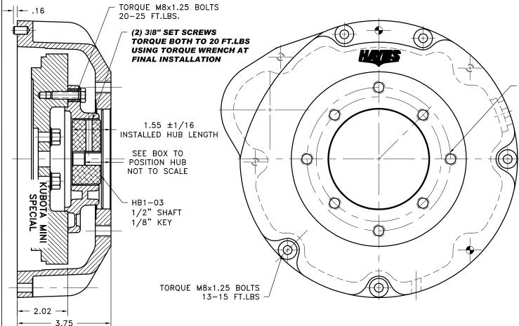
NOTE: REMOVE HUB FROM ASS'Y, PRESET HUB ON SHAFT AS SHOWN. TORQUE BOTH SET SCREWS TO 25 FT.LBS. USING TORQUE WRENCH. SHAFT SHOULD HAVE A MINIMUM OF 3/4" OF ENGAGEMENT IF NOT CONTACT FACTORY FOR RECOMMENDATIONS (231) 879-3372 TO GET HUB PRESET USE THIS EQUATION:
