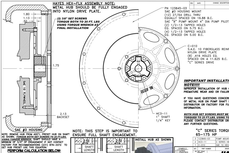
C-010 S.A.E. 10 FIBERGLASS REINFORCED NYLON DRIVE PLATE (8) .416 HOLES EQ. SPACED ON A 11.625 B.C. "C" SERIES DRIVE
