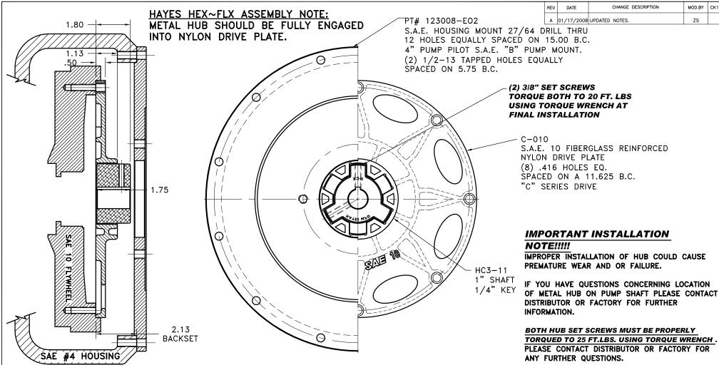
NOTE: REMOVE HUB FROM ASS'Y, PRESET HUB ON SHAFT AS SHOWN. TORQUE BOTH SET SCREWS TO 25 FT.LBS. USING TORQUE WRENCH. SHAFT SHOULD HAVE A MINIMUM OF 3/4" OF ENGAGEMENT IF NOT CONTACT FACTORY FOR RECOMMENDATIONS (231) 879-3372 TO GET HUB PRESET USE THIS EQUATION:
