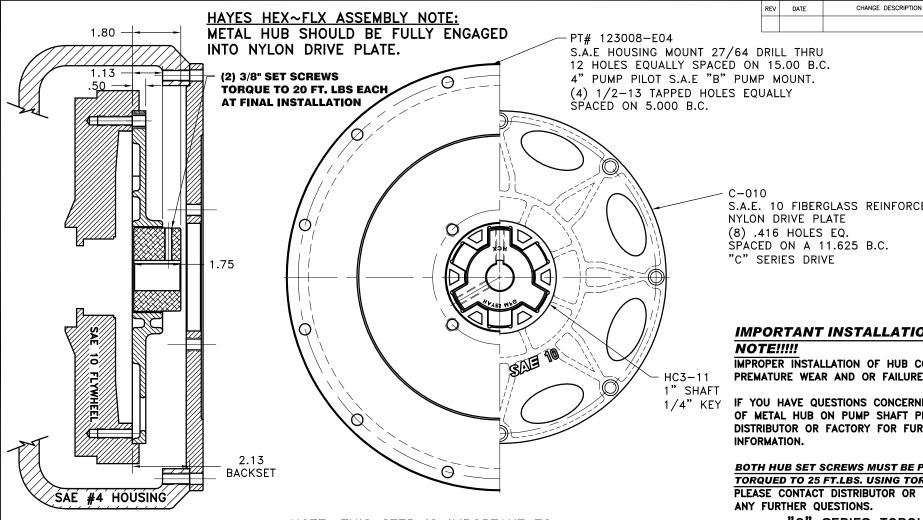
NOTE: REMOVE HUB FROM ASS'Y, PRESET HUB ON SHAFT AS SHOWN. TORQUE BOTH SET SCREWS TO 25 FT.LBS. USING TORQUE WRENCH. SHAFT SHOULD HAVE A MINIMUM OF 3/4" OF ENGAGEMENT IF NOT CONTACT FACTORY FOR RECOMMENDATIONS (231) 879-3372 TO GET HUB PRESET USE THIS EQUATION:
