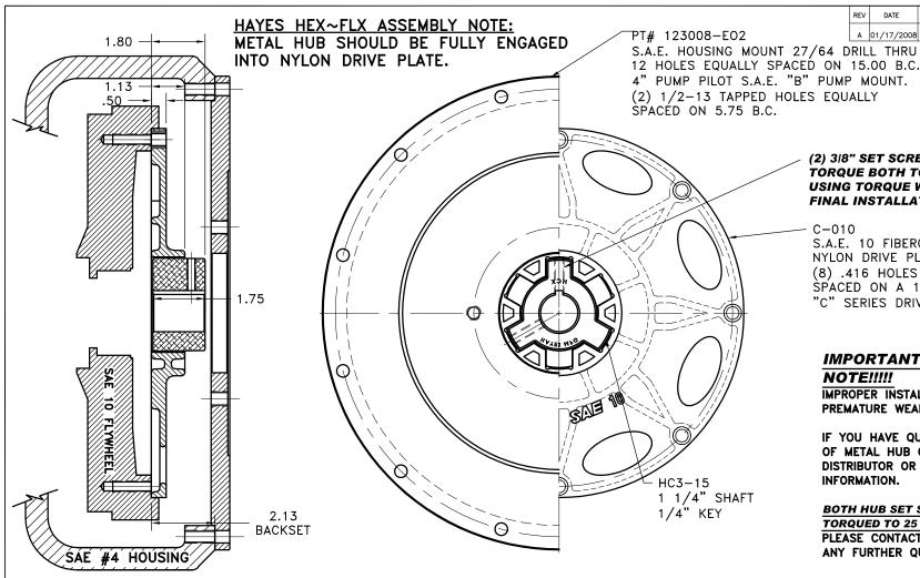
(2) 3/8" SET SCREWS **TORQUE BOTH TO 20 FT. LBS USING TORQUE WRENCH AT FINAL INSTALLATION**
