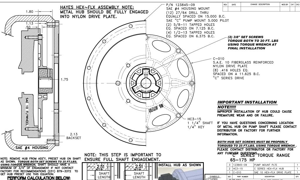
USING TORQUE WRENCH. SHAFT SHOULD HAVE A MINIMUM OF 3/4" OF ENGAGEMENT IF NOT CONTACT FACTORY FOR RECOMMENDATIONS (231) 879-3372 TO GET HUB PRESET USE THIS EQUATION:
