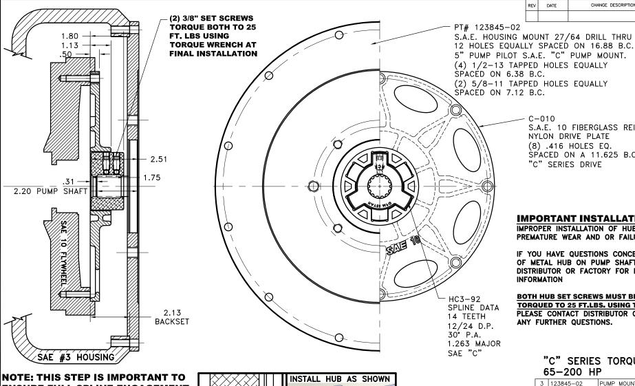
C-010 S.A.E. 10 FIBERGLASS REINFORCED NYLON DRIVE PLATE (8) .416 HOLES EQ. SPACED ON A 11.625 B.C.
