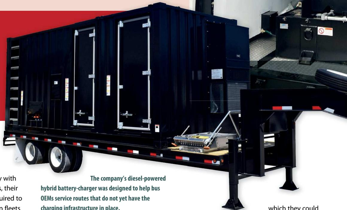
The company's diesel-powered hybrid battery-charger was designed to help bus OEMs service routes that do not yet have the charging infrastructure in place.
