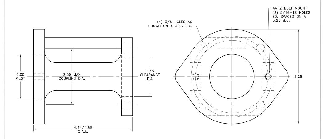
NOTE: UNDERLINED LENGTH DIM. IS STANDARD ANY LENGTH BETWEEN DIMENSIONS CAN BE REQUESTED.
