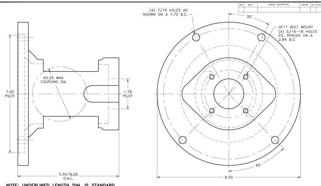
NOTE: UNDERLINED LENGTH DIM. IS STANDARD ANY LENGTH BETWEEN DIMENSIONS CAN BE REQUESTED.
