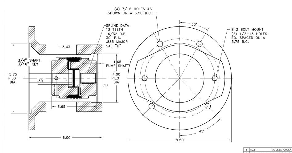
5 G-21-204-6.00 SMALL ENGINE HOUSING 4 300-00-00-M 30 SERIES NEOPRENE INSERT 3 30N-00-00 30 SERIES NEOPRENE INSERT 2 3AO-91-00 30 SERIES COUPLING HALF 1 3AO-07-00 30 SERIES COUPLING HALF DET. PART NUMBER
